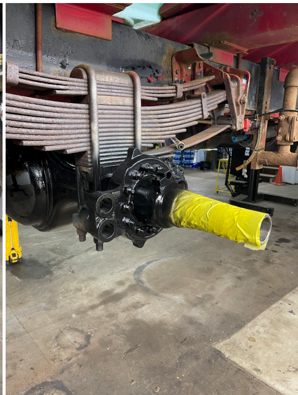
Streets Flush Truck #52488- Reconditioned Rear Axle and New Paint
