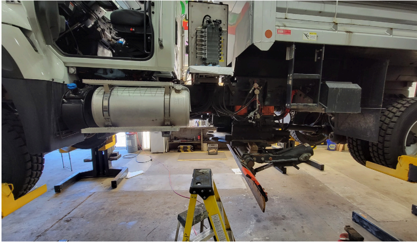
Streets International Plow/Sander #52767- Hydraulic & Front Axle Repair
