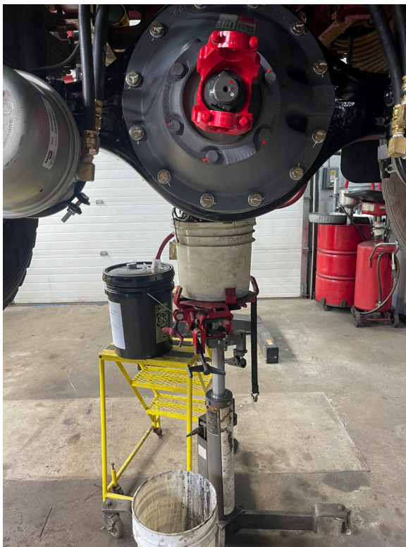
Streets Flush Truck #52488- Reconditioned Rear Axle and New Paint
